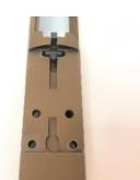
Step 2: Place Outerimpact plate onto slide with notch for the Loaded Chamber Indicator to the front under the cut-out.
